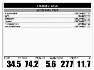
**NOTE:** The speed accessory will be detected only if the paddlewheel has moved since your 1100 Series™ was powered up.
